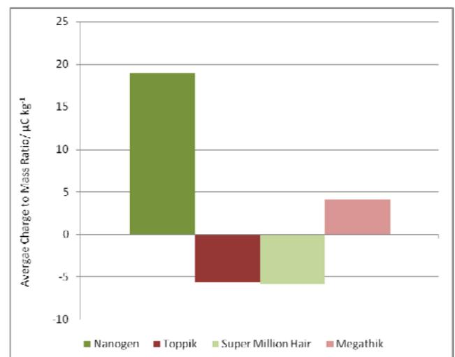
**Figure 2.** Graph to compare the average charge density of various hair building fibre brands after dispensing, over 10 repetitions.
